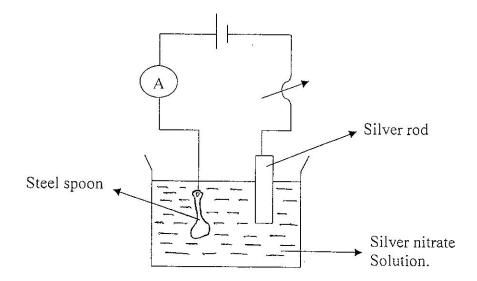
In the apparatus shown above, the electroplating was NOT successful. Identify the **error** in the apparatus set-up then draw the correct set-up in the space below.
