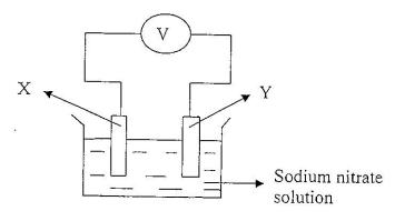
The voltage of different metal pairs were measured and recorded in the table below.
